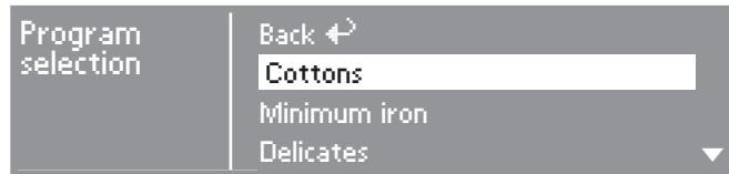
You can use the multi-function selector to select any program. The highlighting will move up or down depending on the direction the multi-function selector is turned in.
